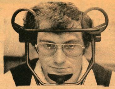
Marc's head is held steady by a bracket to prohibit any exterraneous head movement.
